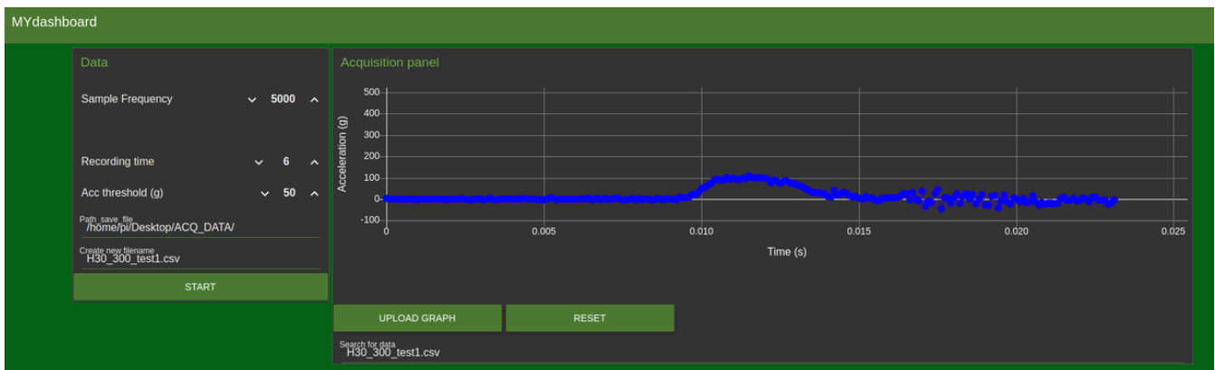
Figure 14: User-friendly dashboard integrated by nodered platform. Data acquisition and saving is automated easing the experiments performance. This dashboard shows one experiment performed with impact velocity of 2.4 m/s ( h = 30 cm) and bumper of R = 300 mm and E = 5 MPa.
